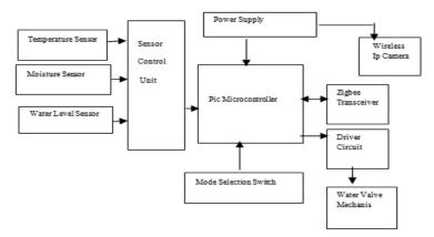
Figure 1: Sensor Control Unit.
