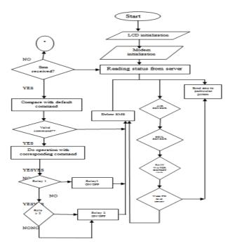
Figure 7: Flow Diagram of Micro Controller.
