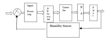
Figure 4: Operation of Humidity Sensor.
